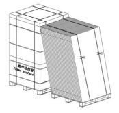
Gently push the module so that it leans against the support, removing the vertical strip of plastic steel
