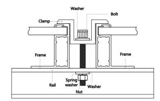
Figure 7. Specific installation of clamps
