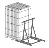
Place a support bracket on either of the recline surfaces of the assembly and remove the three transverse steel strips from the upper part of the assembly with
