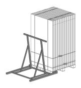
Two people stand on the frame surface of the module to hold the component, while the other person cuts the lower two transverse plastic steel packing belts
