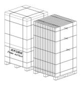
Use scissors to remove the three transverse steel strips from the upper part of the assembly
