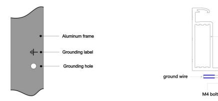
Figure 1. Ground hole and its identification
